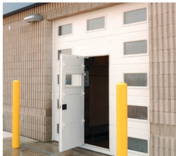
A pass door is an entry door that is built into the garage door, allowing for entry and exit without having to open the garage door. Available in 2" sandwich. Note: Doors are not ADA or egress compliant. Minimum of 15" of headroom is required.
