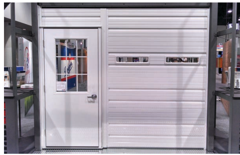
A wicket door is an entry door permanently mounted next to a garage door in the same opening. The whole assembly can then swing open, allowing the entire width of the opening to be utilized. Available in any commercial model. Note: Doors are not ADA or egress compliant. Minimum of 24" of headroom is required.
