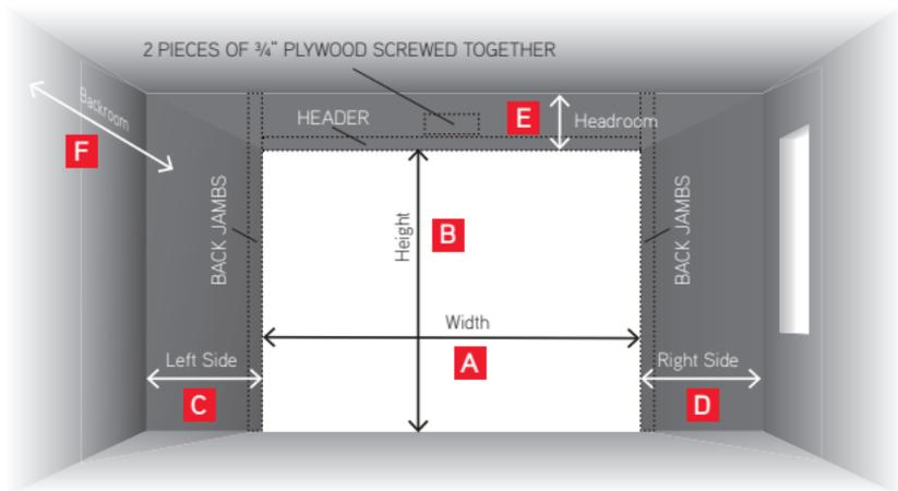
1) Measure existing door opening's width **A** and height **B** in feet and inches. This determines the size of door needed. Never base your measurements on the size of the existing door but on the door's opening instead.
